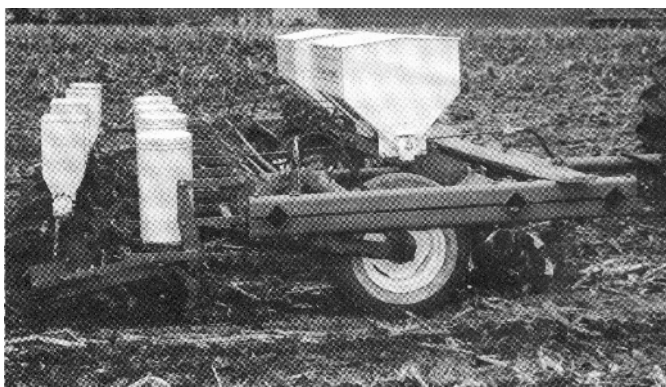
The wavy coulters were adopted to do row tillage on this 1960s Allis Chalmers “no-till” planter.
